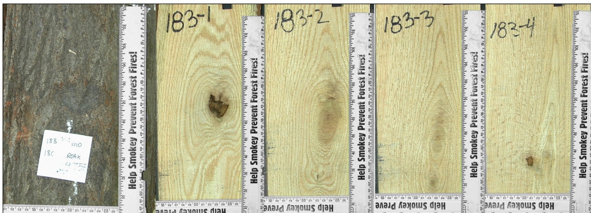
Figure 2. Surface indicator and internal defect slices for a medium distortion defect from a red oak log.
