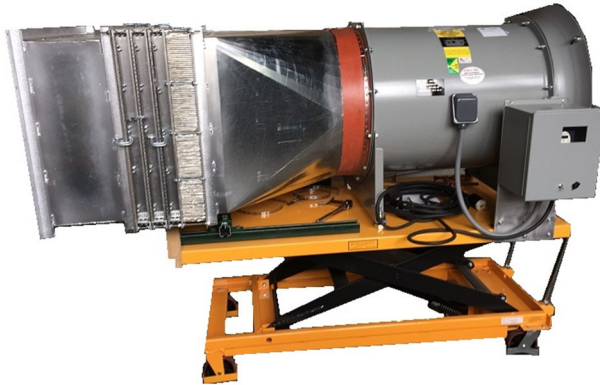
Figure 1. Wind generator designed at FPL with a continuously variable velocity from 0.1 m/s to 6 m/s.
