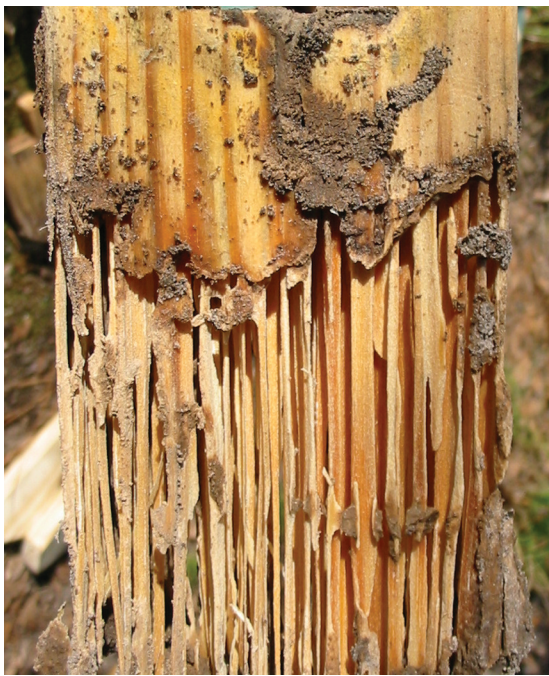
Fig. 2. Damage to untreated wood caused by termites after only six months of soil contact in Louisiana. Courtesy of Stan T. Lebow and the U.S. Forest Products Laboratory.
