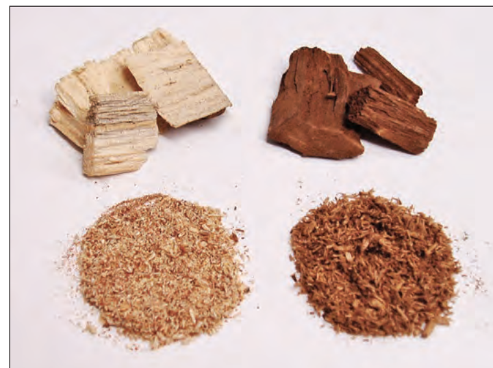
The dark chips have undergone hot water extraction; they are then ground and ready to be further processed into bioplastics.
