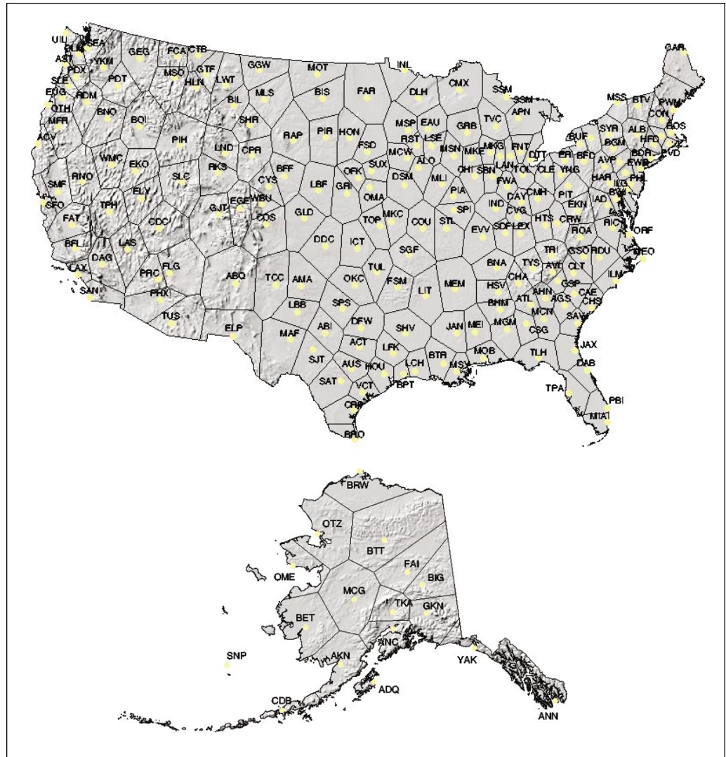
Figure 7—Neighborhoods for determining local inversion potential in the contiguous 48 states and Alaska. Letters indicate the National Weather Service identifier for the station that was used to determine calm, clear conditions within the neighborhood, and the yellow dot shows its location.
