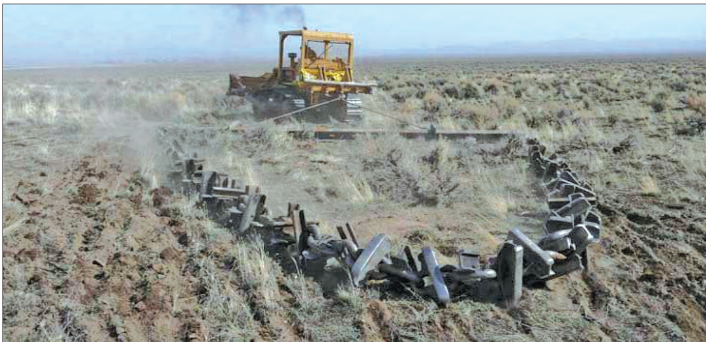
Chain harrow used to partially reduce sagebrush near Rush Valley, Utah.
