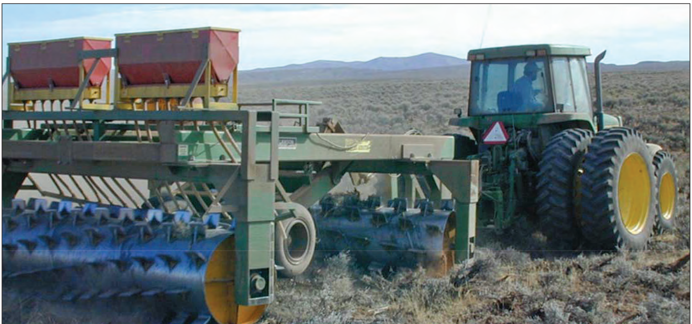
Meadow aerator-seeder planting seeds while aerating the soil near Evanston, Wyoming.
