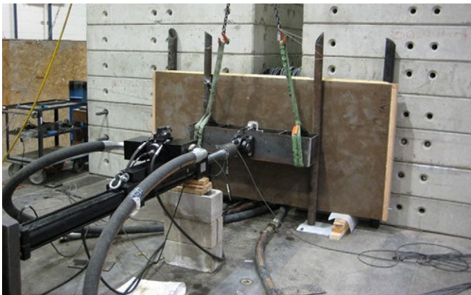
Figure 17. BioSIPs prototype undergoing transverse bending test using a 22-kip MTS actuator.
