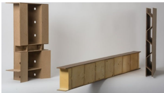
Figure 7. BioSIPs structural panels for wall, floor and roof constructions. Left to right: noninsulated panel core with electrical perforations and conduit channels, and without panel surface skins; insulated panel section with exterior surface skins; panel section with skins and without insulation.
