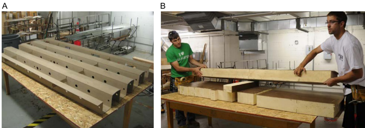
Figure 5. (A) and (B). Full-scale BioSIPs 3D panel core with holes for addition of electrical conduit and wiring. BioSIPs with insulation encapsulating 3D cores, and including panel skins, being stacked by team members for shipment.
