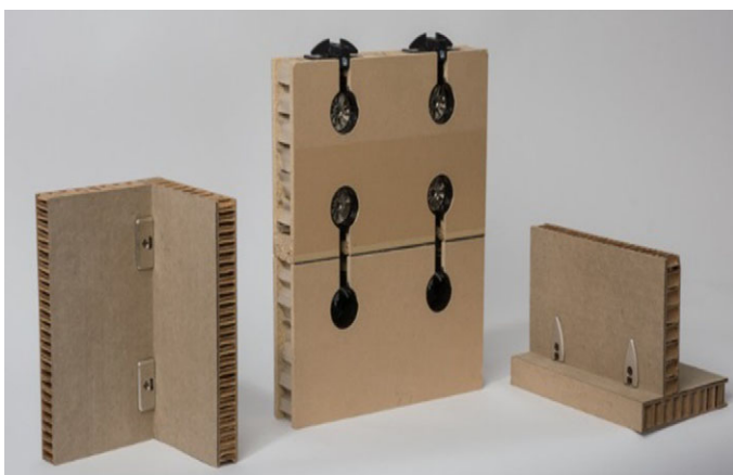
Figure 22. State-of-the-art attachment systems joining dense, thin bioboard for the construction of BioSIPs furniture and interior systems.
