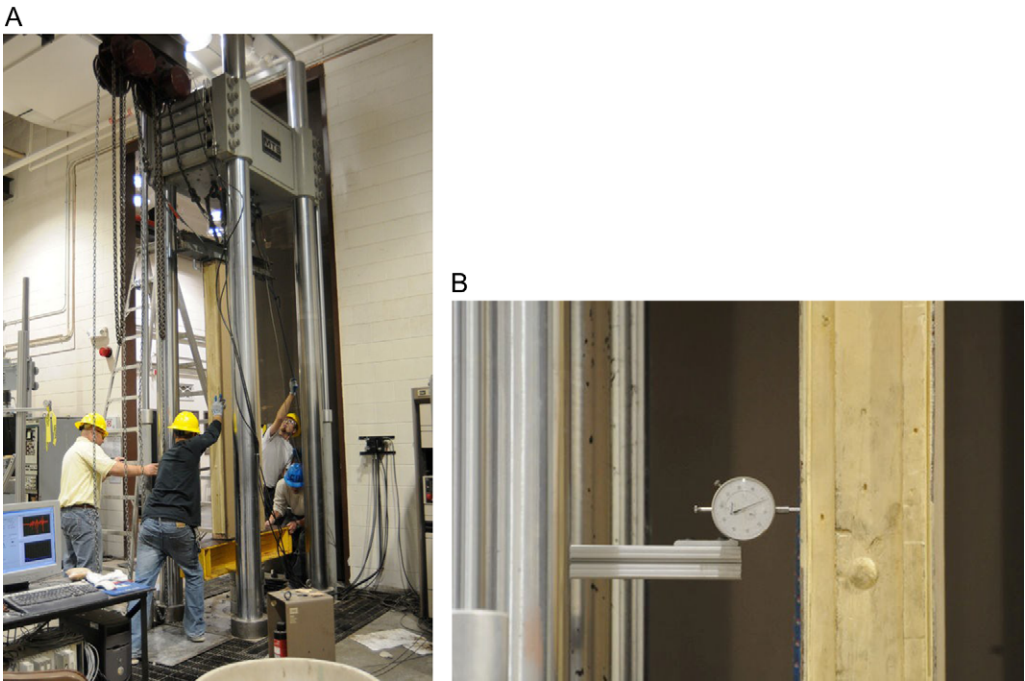
Figure 16. (A) and (B). Axial testing sample of BioSIPs being placed in a 1000-kip MTS actuator (universal testing machine) by team members. Dial micrometer measuring BioSIPs deflection during testing.
