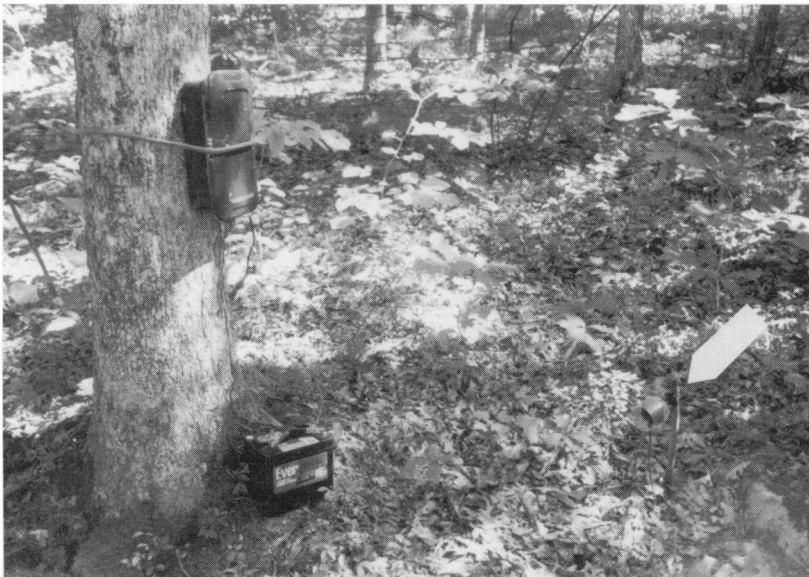
Figure 1. The transmitter in its case is fastened to a tree (left) with the battery below it, and the camera in its waterproof housing is to the right (arrow). All 3 components would be covered in camouflage cloth when in use, and the transmitter and battery would be placed 5–10 m from the camera and nest.
