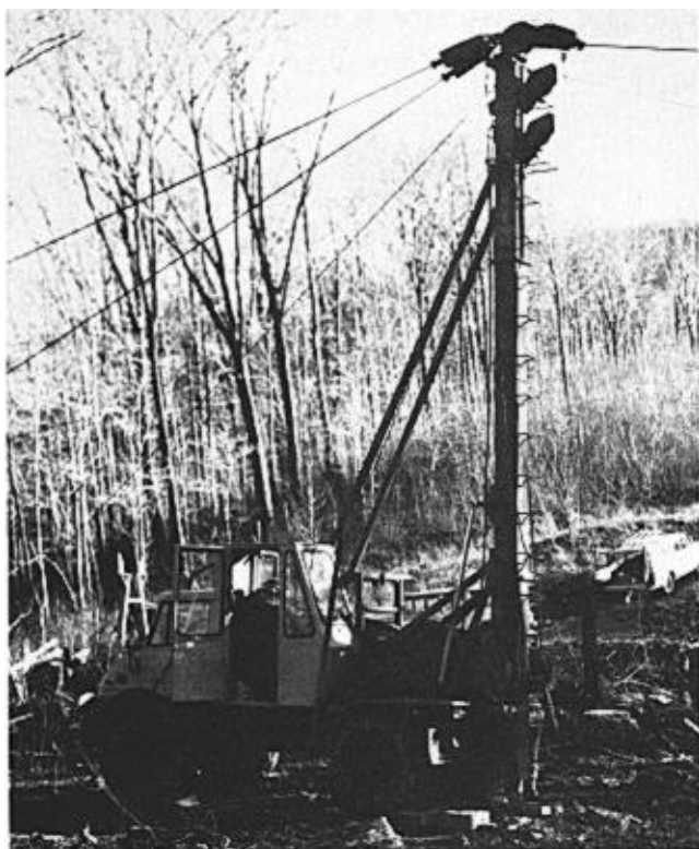
Figure 2. URUS 1000-3 yarder mounted on Mercedes-Benz Unimog truck as tested in this study.
