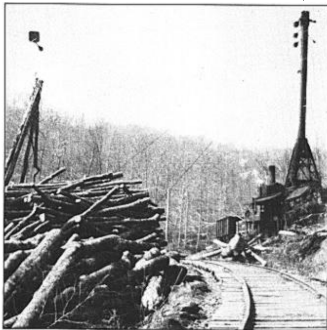
Figure 1. Steam-powered cable system logging hardwoods in West Virginia—the type of system used extensively in early 1900's.
