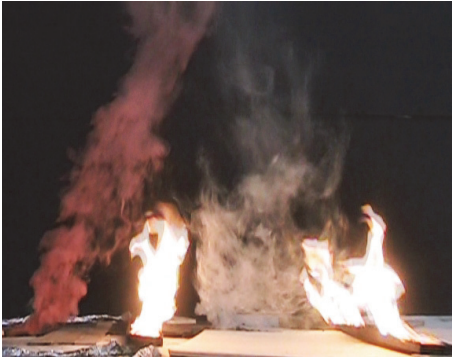
FIGURE 8: Use of smoke cartridges for flow field visualization. Exaggerated flame angle on right is fictitious, due to perspective distortion (figure is cropped; camera is actually centered on left fire).
