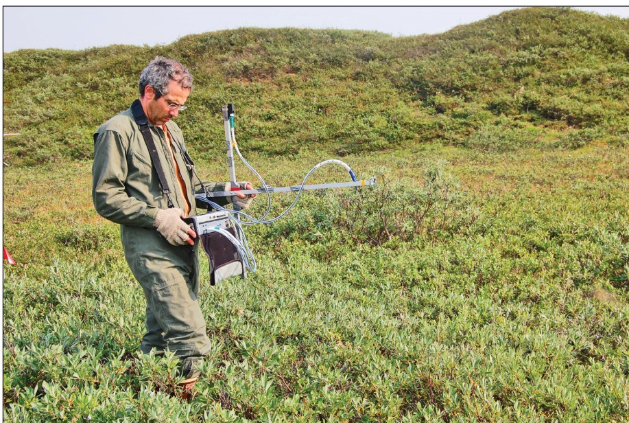
Robert Pattison makes ground-based measurements of the surface normalized difference vegetation index (NDVI). These data were compared to satellite NDVI measurements.
