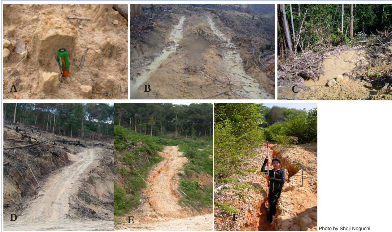
Figure 3. Erosion features in Bukit Tarek: (A) pedestal erosion features, (B) overland flow on the logging road, (C) sediment deposition by forest buffer, (D) skid trail just established (ca. Jan 2004), (E) skid trail six months following logging, (F) skid trail 13 months following logging.
