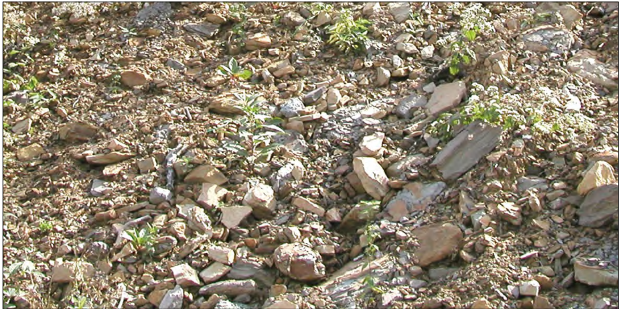
Figure 2-2.—A mixture of weathered brown and unweathered gray sandstones, loosely graded to form a soil medium suitable for trees in West Virginia. Photo by J. Burger, Virginia Tech, used with permission.
