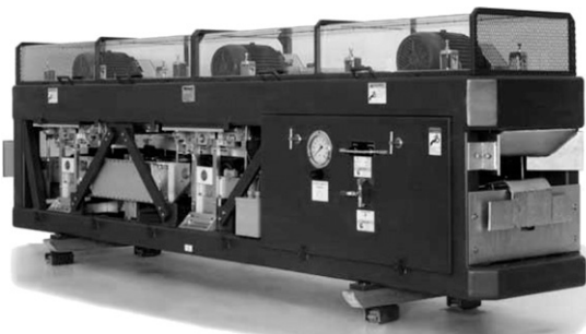
Figure 1. Continuous proof bending evaluation: Mobile High Capacity Lumber Tester Model 7200.
