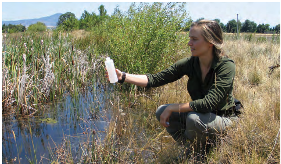
Figure I.3 —Nursery water needs to be tested for pH, salinity, pesticides, and the presence of fungi, nematodes, insects, and weed seeds, especially if a river, pond, or reservoir is the water source. Photo by Thomas D. Landis, USDA Forest Service.
