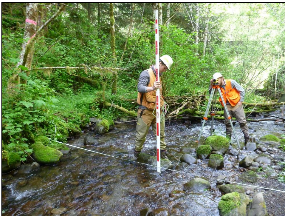
Figure 2-5. Sampling bankfull depth using a stadia rod and auto level.
