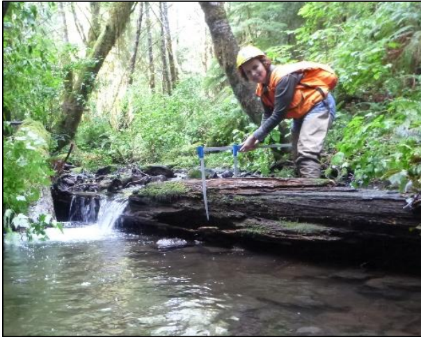
Figure 5-4. Measuring diameter (a) and length (b) of in-stream large wood.
