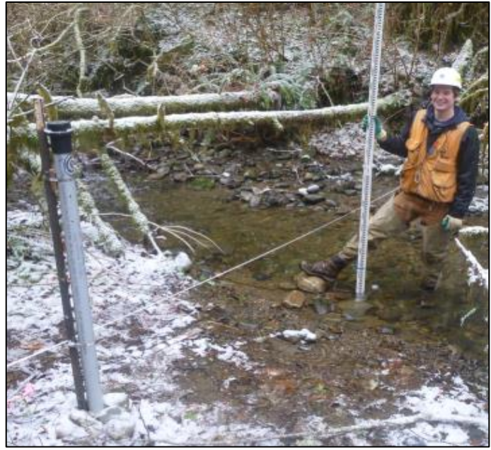
Figure 8-9. Example of a fixed-point for staff gage measurements when no anchor for a vertical installation of a staff gage is available: a) end cap of a recording gage housing is used as fixed measurement point; b) taking a measurement with unfixed staff gage.
