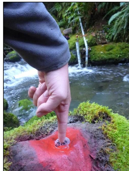
Figure 8-16. Gage Reference Point installed on large stable boulder near recording gage.
