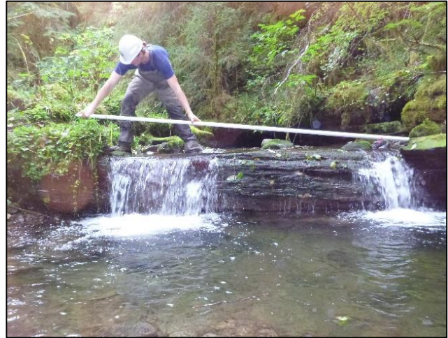
Figure 5-4. Measuring diameter (a) and length (b) of in-stream large wood.
