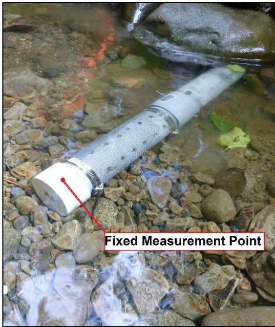
Figure 8-9. Example of a fixed-point for staff gage measurements when no anchor for a vertical installation of a staff gage is available: a) end cap of a recording gage housing is used as fixed measurement point; b) taking a measurement with unfixed staff gage.
