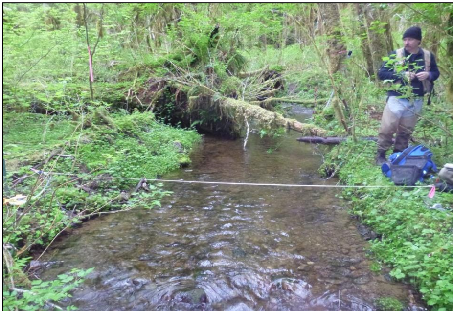
Figure 8-10. Discharge measurement transect with measuring tape anchored above wetted surface.
