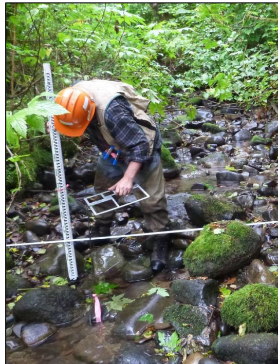
Figure 4-4. Sampling channel substrate using the stadia rod and gravelometer.
