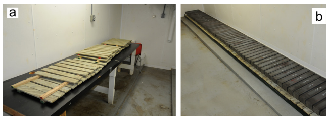
Figure 2—Plywood specimens in a humidity- and temperature-controlled chamber: (a) unloaded specimens; (b) specimens loaded with 40-lb weights.
