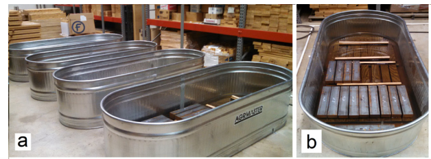
Figure 5—Tanks containing submersion plywood specimens: (a) all tanks in the temperature- and humidity-controlled chamber; (b) layout of submersion unloaded (SU) and submersion loaded (SU+L) specimens in the tank.
