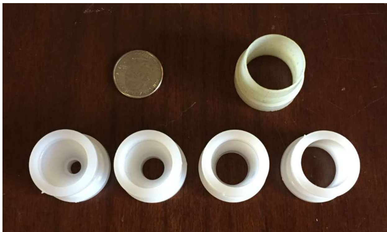
Figure 1. Alternative sample cups for XRF analysis. From left on bottom row: 6mm, 10mm, 15mm and 20mm aperture. Top row shows American quarter and standard (24mm) Asoma cup.
