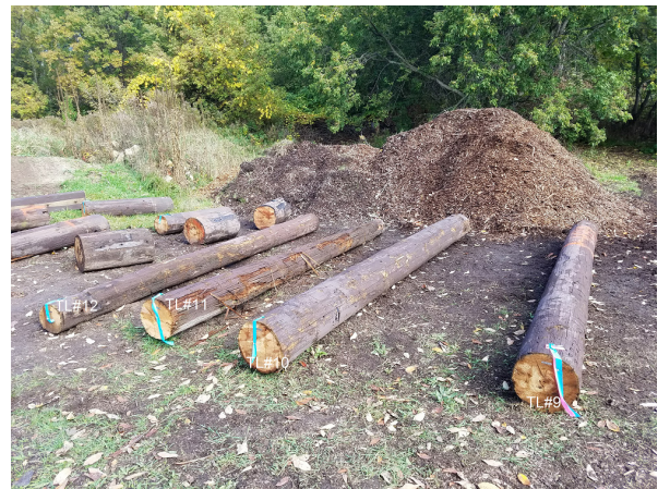
Figure 5. Timber sections TL#9 through TL#12 were the middle section of the tower's legs.
