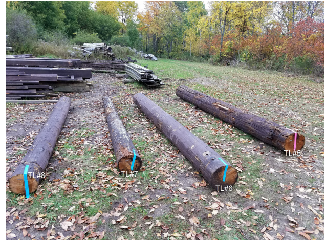
Figure 4. Timber sections TL#5 through TL#8 were from the uppermost portion of the tower's legs.
