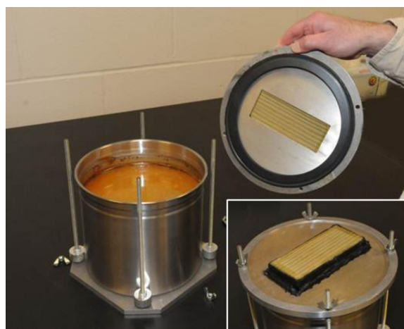
FIG. 2 Cup used in the vapor diffusion test. The lid was sealed with a gasket held down with threaded rods. The edges of the sample were sealed with butyl tape (inset).
