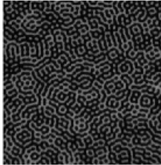
FIGURE 5 Laser printed digital image correlation pattern on specimen, 25 mm × 25 mm region
