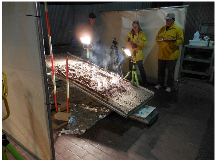
Fig. 1. Experimental bed setup including (a) diagrammatic of sections (from Heinsch et al., in press); and (b) photo of burn bed. In experimental setup, yellow circles represent the halogen lights; purple triangle is position of video camera; hatched zone represents ignition zone consisting of pine needles and excelsior; gray boxes on each end indicate the scales to measure mass loss. Gray rings are the stadia rods used to measure flame height and rate of spread. (For interpretation of the references to color in this figure legend, the reader is referred to the web version of this article.)
