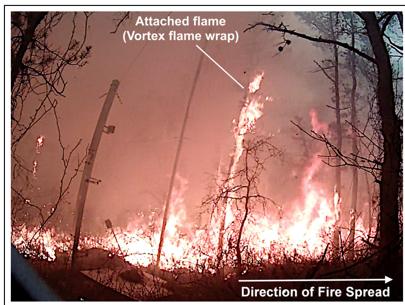
Figure 13. Still shot from video camera at plot X showing tree trunk with wind vortex flame wrap.
