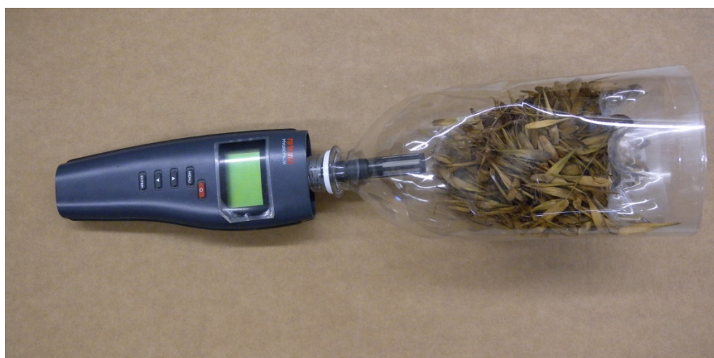
Figure 3—A hygrometer is used test whether the seeds are sufficient dry for long term storage.
