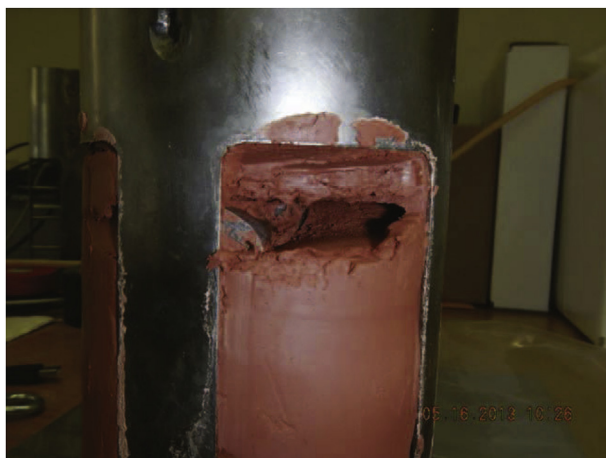
Fig. 6. Photograph of the clay following the LCBR operation. The exposed impeller blade was moving right to left. A cavity is apparent behind the blade. The space in front of the blade is filled with clay because an impeller blade below (not visible) pushed material into the previously formed cavity.
