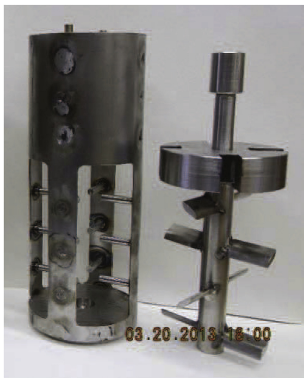
Fig. 2. Photograph of the LCBR insert and impeller, designed to fit in a 2 L Parr reactor. Left: the cylindrical insert with interior static pin array. Right: the bladed impeller shaft with the slotted weight and Parr shaft coupling.
