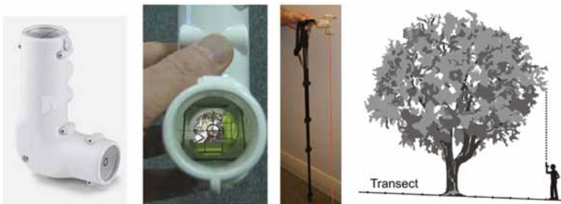
Figure 4 —Densitometer (left two panels) and laser sampling device (panel 3) for measuring presence of vegetation along a vertical line at each point along transects (panel 4).
