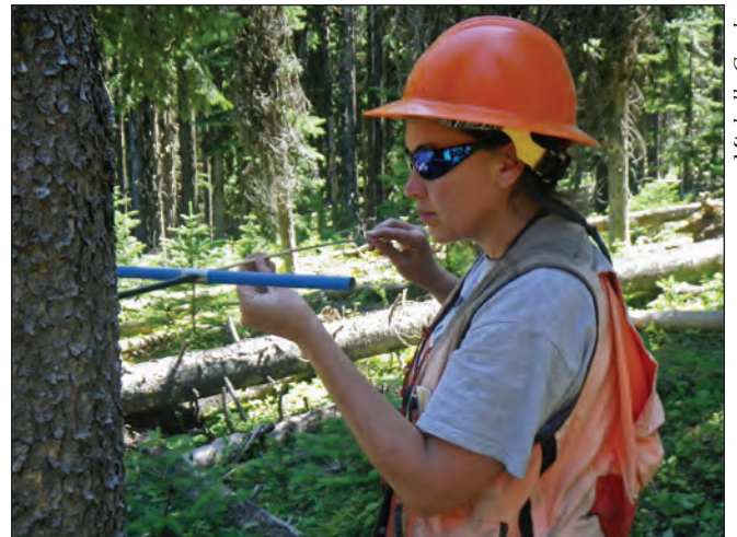
Figure 20—Field crew collecting an increment core to estimate age and growth rates.
