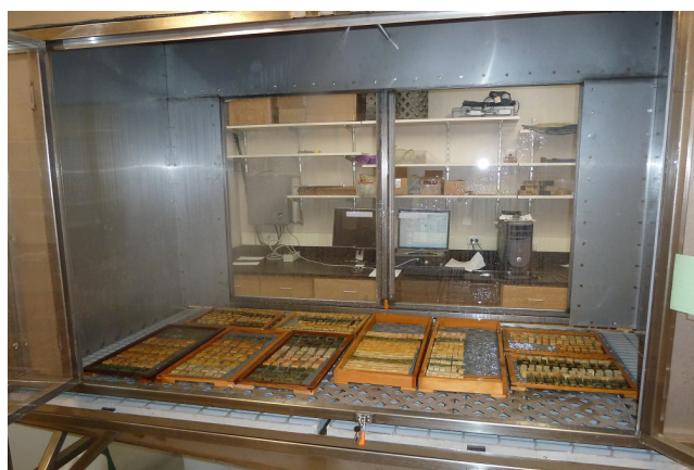
Figure 3. Device used to subject specimens to leaching with simulated rainfall.
