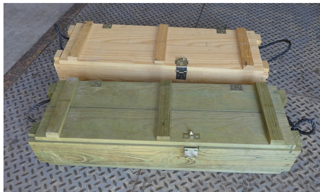
Figure 1. Nailed ammunition boxes are one example of durable wood packaging materials that are dip-treated with preservative.
