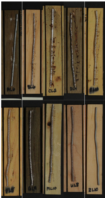
Figure 16. Bottoms of wires after the 8-week exposure. Dip formulations from left to right. Top row: CuC, AzI, pCuA-1, sCuA, Cu8-1. Bottom row: Cu8-2, CuN, pCuA-2, water, ZnN.
