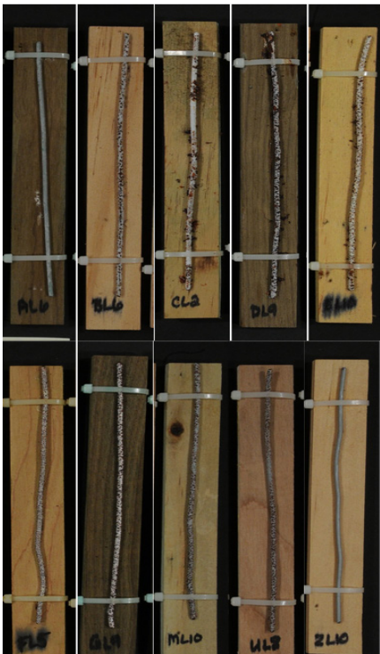
Figure 15. Tops of wires after the 8-week exposure. Dip formulations from left to right. Top row: CuC, AzI, pCuA-1, sCuA, Cu8-1. Bottom row: Cu8-2, CuN, pCuA-2, water, ZnN.
