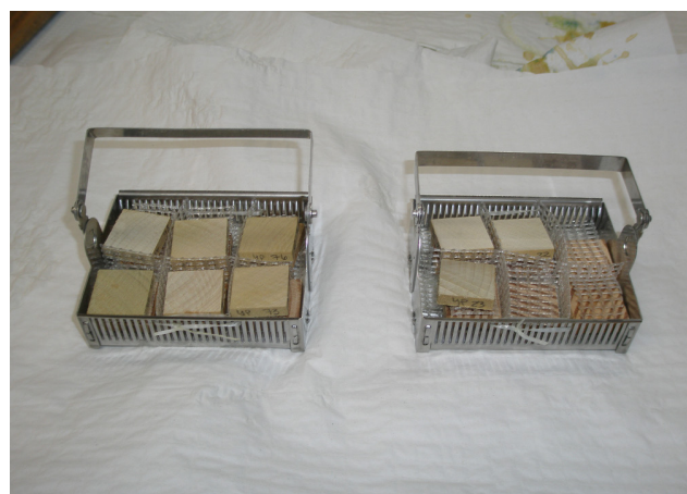
Figure 4. Termite specimen preparation for dip treatment.
