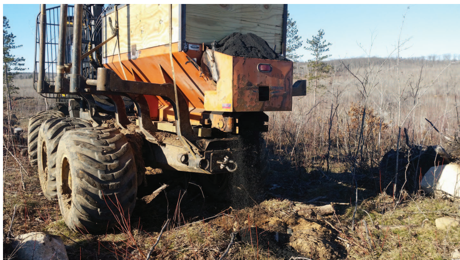
Figure 2. Modified skidder with spreader used for broadcast wood ash application.
