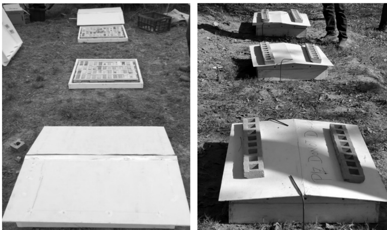
Figure 1. Ground proximity test (AWPA- E26) set up in USA (left) and Pakistan (right).
