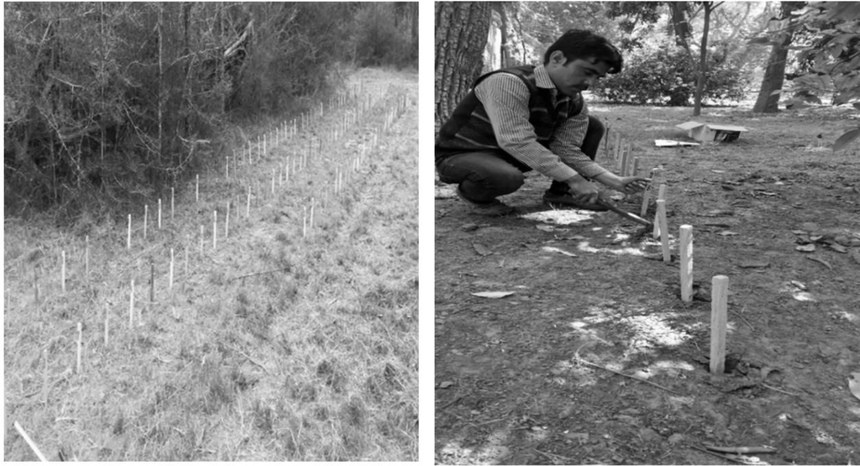
Figure 2. Field stake test (AWPA- E7) set up in USA (left) and Pakistan (right).
