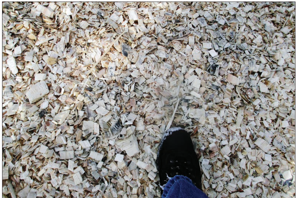
Figure 7—Aspen wood chips used for cofiring, showing uniform size and composition as well as lack of bark, foliage, or contaminants.
