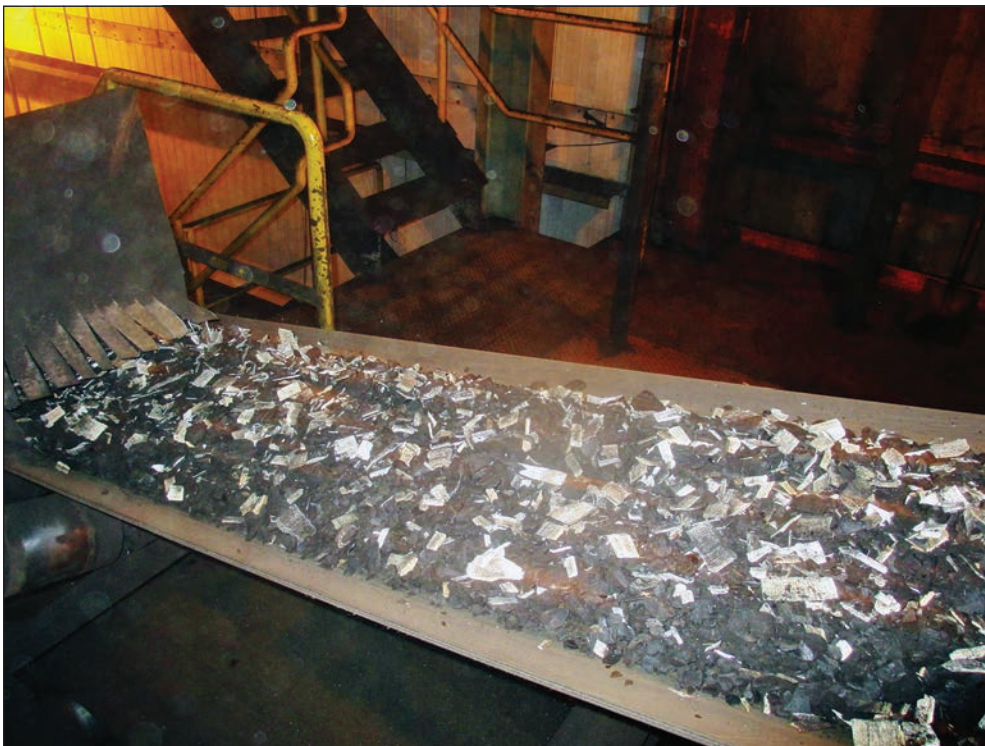
Figure 6—Fully mixed wood chips (white) and coal (black) mixture travelling on a conveyor belt before entering the combustion chamber.
