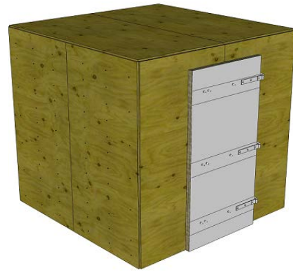
Figure 3. Safe room with plywood nailed and glued to lumber beams.
