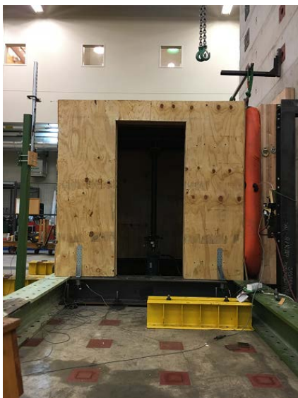
Figure 29. Lateral wind pressure test setup using an airbag. Airbag is orange.
