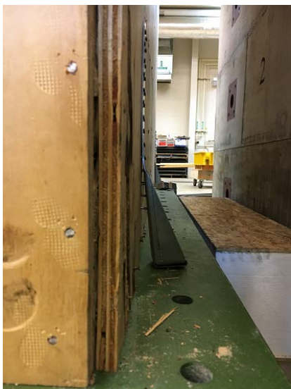
Figure 35. Nail pullout of tie-down at two times design load.
