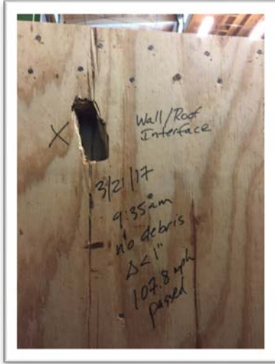
Left: exterior damage after impact; Right: interior damage after impact. (impact location: 29 in. left of center, 7 in. below top center of room side.)
