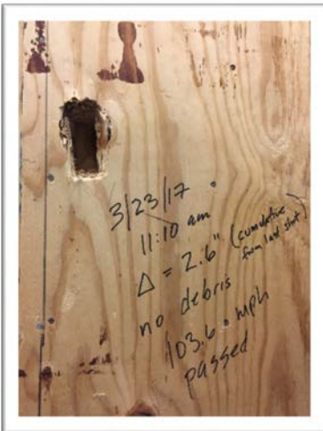
Left: front of room after impact test; Right: back of panel after impact test. (impact location: 3 in. right of center, 27.5 in. down from top.)
