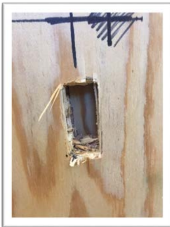
Left: front of panel penetration; Right: slight cracking on backside of panel.
