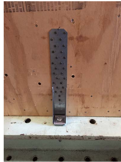
Figure 19. Tie-down anchor nailed to safe room and bolted to steel beams that were clamped to test floor.
