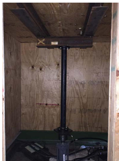
Figure 36. Hydraulic ram and steel tree to load safe room roof.
