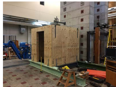
Figure 20. Tie-down of safe room to strong floor.
