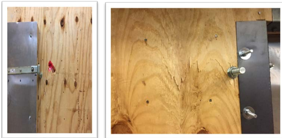
Left: front of panel after impact test; Right: back of panel after impact test.
