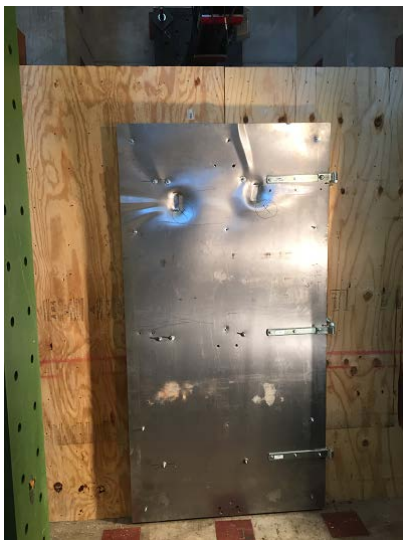
Figure 10. Door impact damage.
