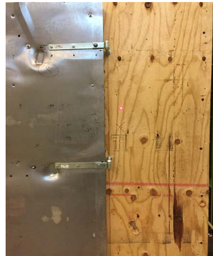
Figure 11. Impact location adjacent to door opening (target is red laser dot midway between the two hinges and slightly to the right).
