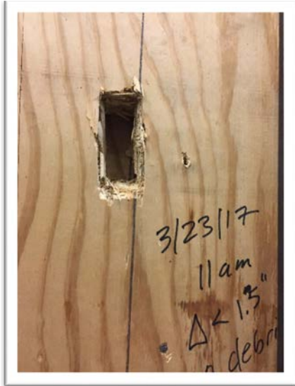
Left: front of room after impact test; Right: back of panel after impact test. (impact location: 32 in. right of center, 16 in. down from top.)
