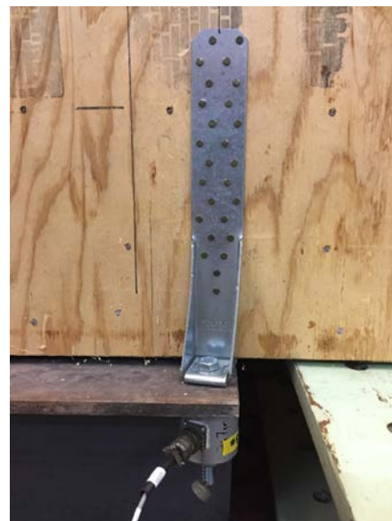
Figure 34. Bending of tie-down at two times design load.
