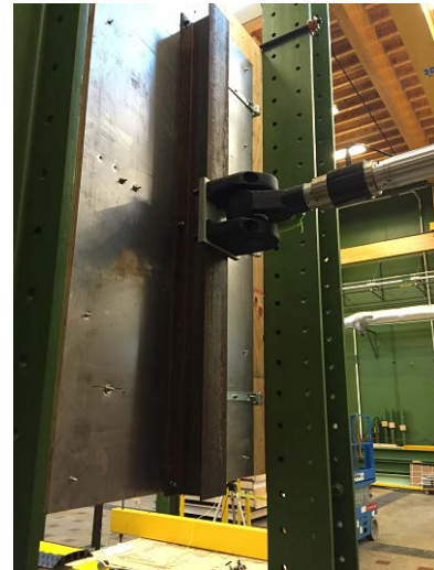
Figure 27. Door suction test.
