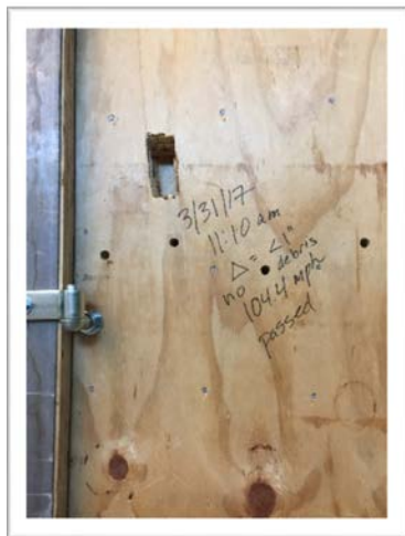
Left: front of room after impact test; Right: back of panel after impact test. (impact location: 18.5 in. down, 20.5 in. left of top right corner.)
