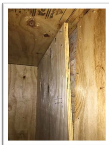
Left: front of room after impact test; Right: back of panel after impact test. (impact location: 3 in. right of center, 27.5 in. down from top.)
