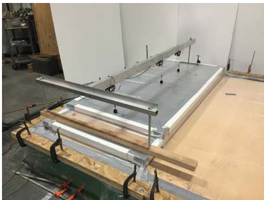
Figure 26. Door wind pressure test.
