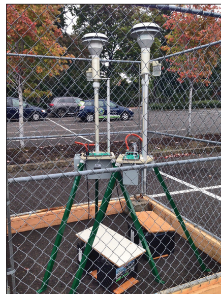
After the moss study team found high levels of cadmium in moss in southeast Portland, the Oregon Department of Environmental Quality set up this air pollution monitor near the hotspot.
