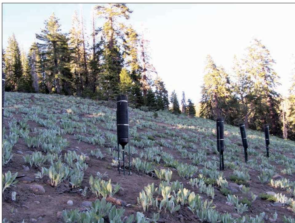
Figure 3.21—Ion exchange resin bulk deposition collectors located in forest clearings. Because of potential bird contamination, it is recommended that five to six replicate samplers be used in most open-site locations.
