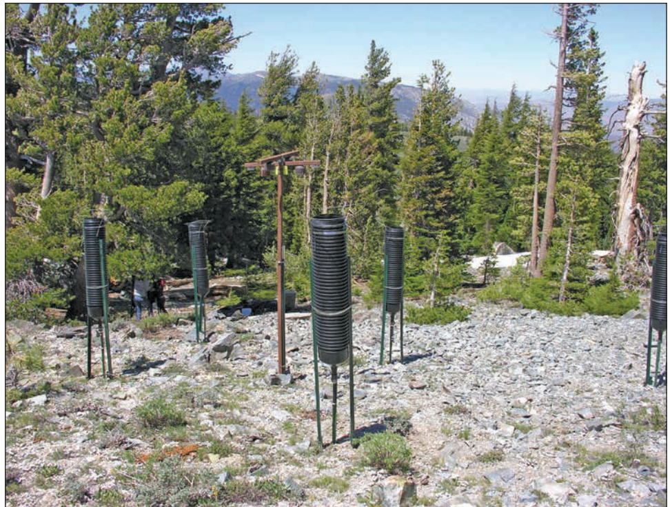
Figure 3.14—Ion exchange resin bulk deposition samplers installed in a forest clearing and next to a pole containing a suite of passive samplers. Throughfall collectors are also being installed under trees in the adjacent forest stand.
