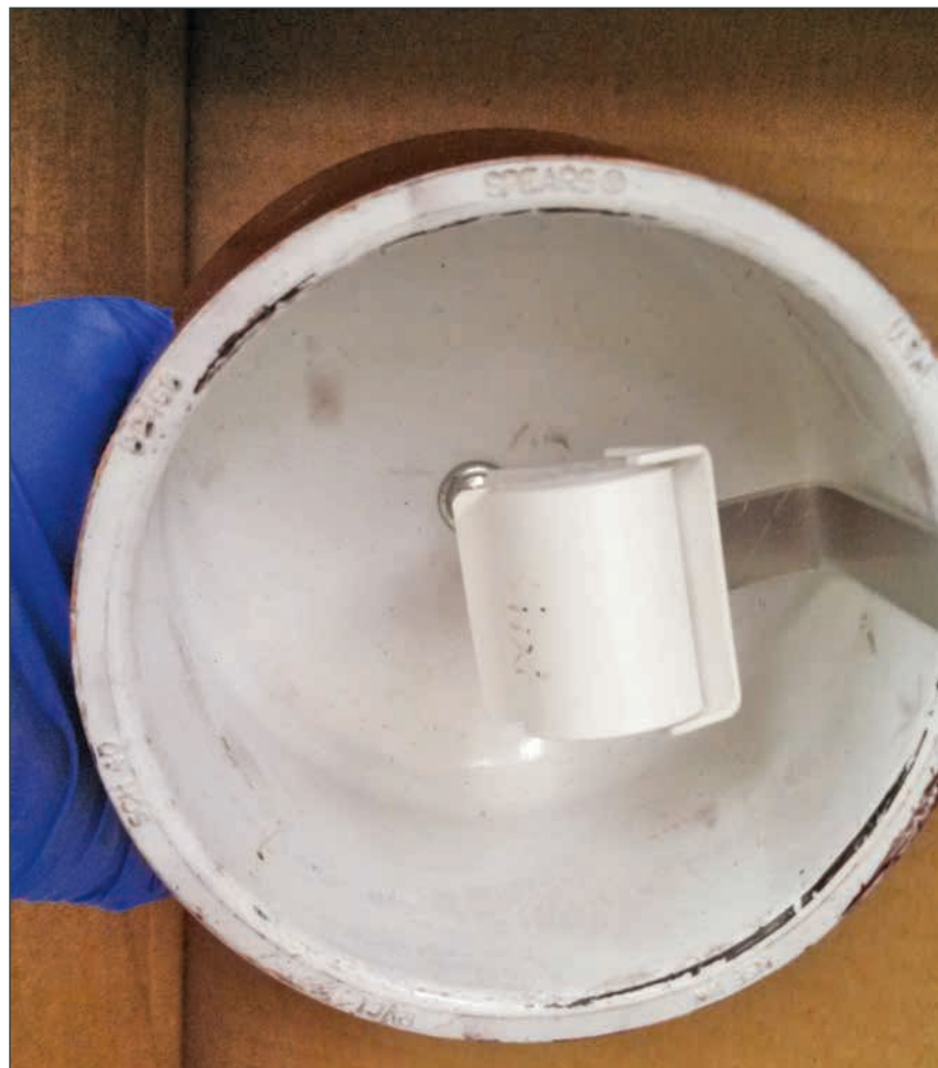
Figure A1.16—Ogawa sampler positioned correctly in the shelter.
