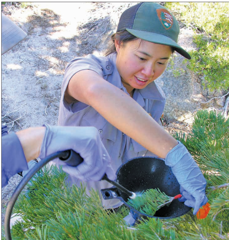
Figure 4.1—Rinsing of foliage on tree branches to measure the ions in the collected rinse solution that were atmospherically deposited to the branches. From this, deposition fluxes since the time of the previous branch rinsing can be calculated.
