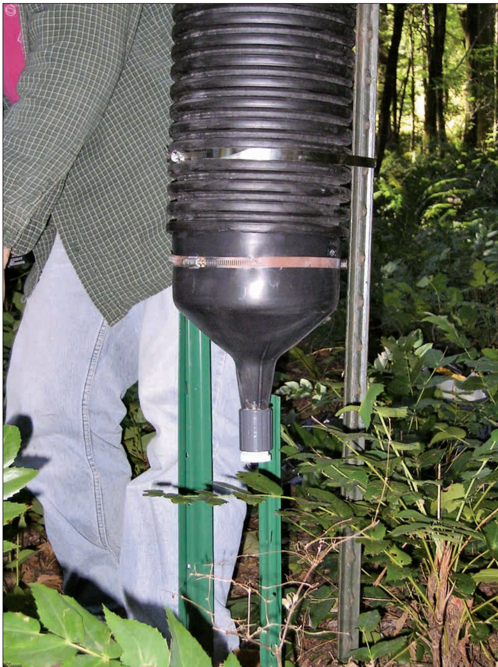
Figure 3.7—An ion exchange resin (IER) sampler with snow tube attached. Notice that the IER column is not yet attached to the bottom of the sampler. A new IER column is attached at the beginning of each new exposure period, typically for 5- to 6-month intervals.
