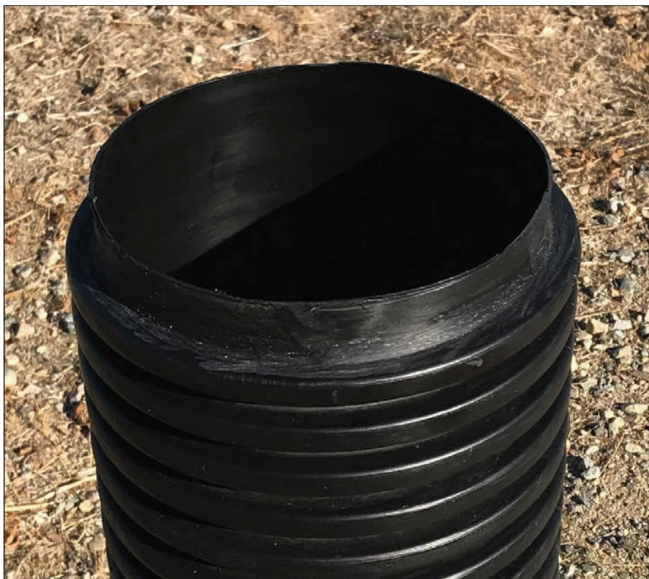
Figure A2.1—Side view of the top (upper end) of a snow tube. The top outer corrugated ring has been ground off from the tube to provide a thinner wall at the snow tube opening.
