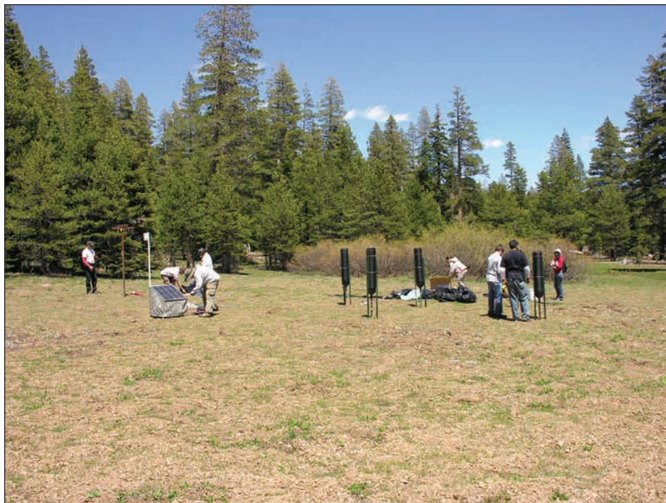
Figure 3.8—Installation of ion exchange resin bulk deposition samplers in a forest clearing in the Lake Tahoe basin. Passive samplers for gaseous pollutants and a battery/solar-powered active ozone monitor (Burley et al. 2015) were also installed at this study site.
