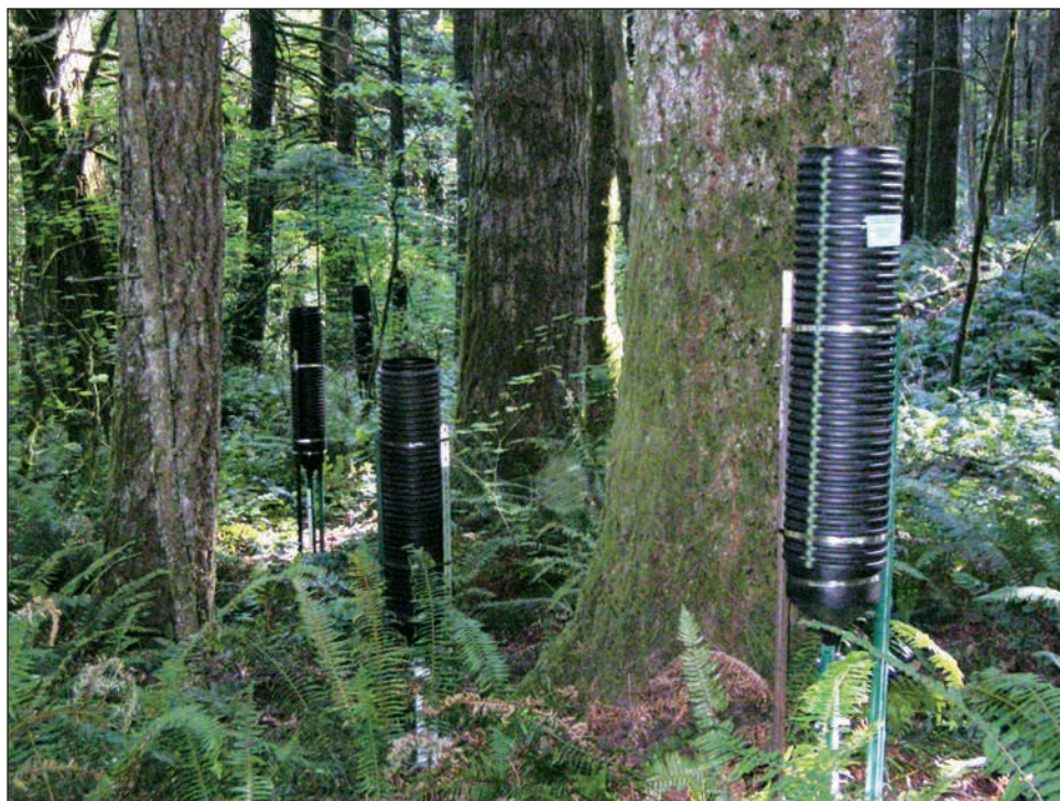
Figure 3.12—Ion exchange resin throughfall collectors with snow tubes attached, installed at a predetermined spacing along a transect at a forest site.
