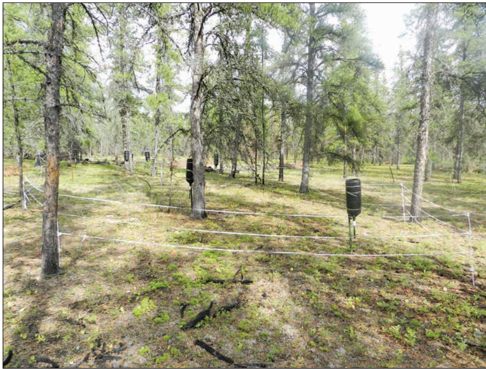
Figure 3.19—Ion exchange resin throughfall collectors and snow tubes in an area protected from bear damage by an electric fence. The need to circumscribe the monitoring area with an electric fence restricts the size of the potential monitoring site.
