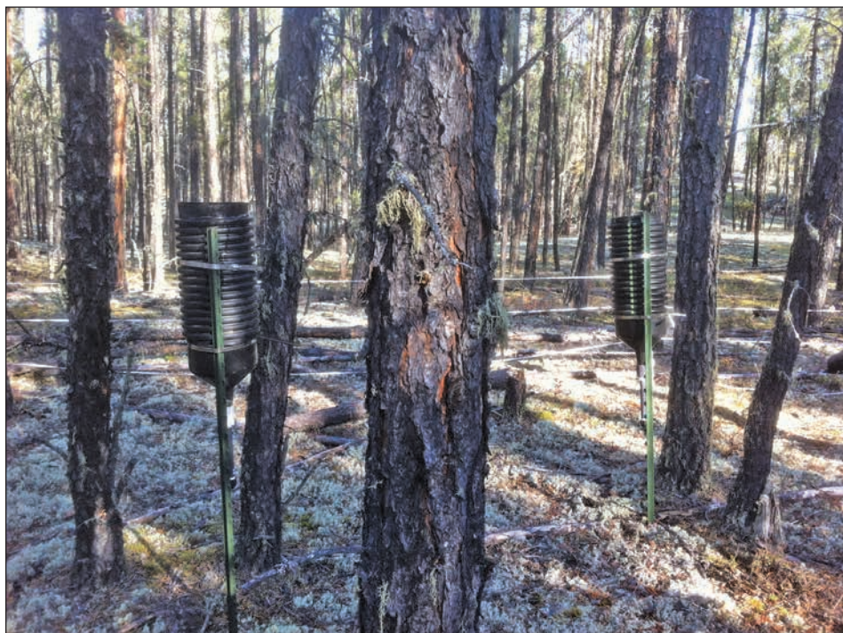
Figure 3.16—View of two ion exchange resin throughfall collectors in a jack pine ( Pinus banksiana Lamb.) stand in northern Alberta, Canada, with shorter (0.5 m) snow tubes installed in a stand with low snowfall volumes.
