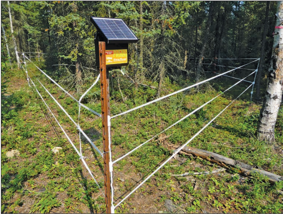
Figure 3.18—In areas of high bear activity, the only effective solution to prevent disturbance of the ion exchange resin collectors is to install solar-powered electric fences around the area where the collectors are located.
