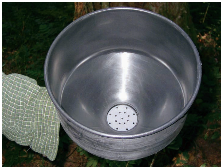
Figure 3.4—Inside view of a funnel used for monitoring throughfall or bulk deposition with ion exchange resin (IER) collectors. The disk in the center of the funnel is to keep coarse litter out of the IER columns. Polyester floss is also inserted on the top of the IER column as a fine filter.
