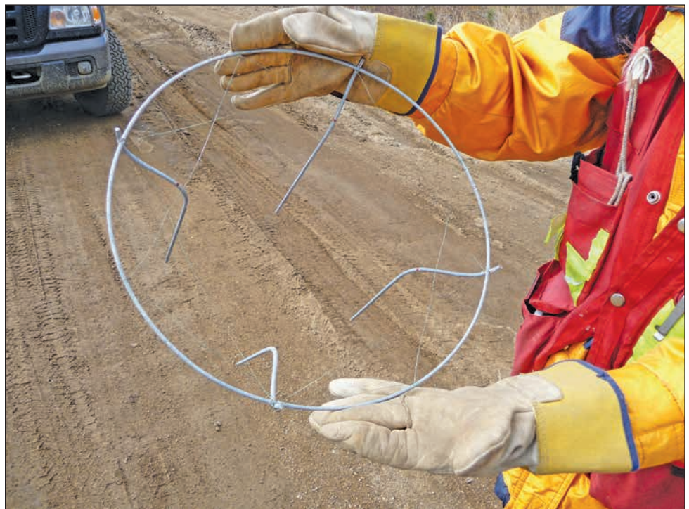
Figure 3.20—Example of a simple bird sitting ring made from a tomato cage prior to placement on a funnel or snow tube. Fishing line has been strung across the ring to further deter birds from perching on the collectors.
