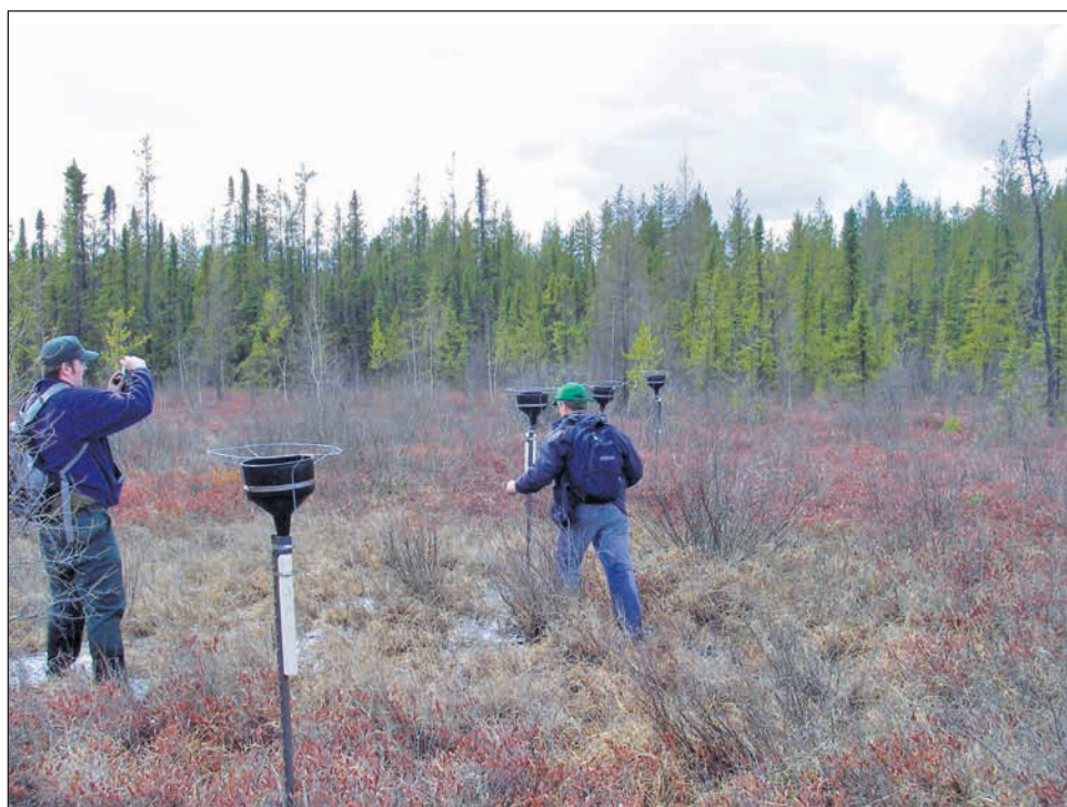
Figure 3.9—Bulk deposition ion exchange resin (IER) samplers being installed in a bog, a natural forest clearing, in a remote boreal forest site in northern Alberta, Canada. Notice the bird rings installed on the funnel collectors to discourage birds from perching on the funnels. The white tubes function as a shade covering over the IER columns, to prevent direct sun exposure of the IER columns.
