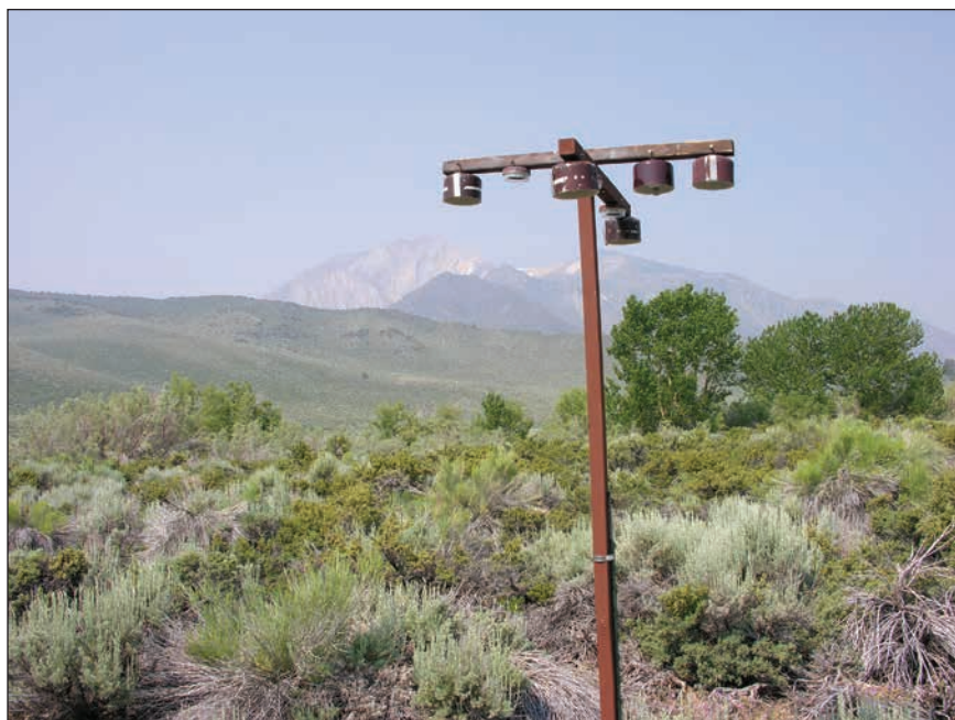
Figure 2.4—Multiple passive samplers installed at a single field site in the White Mountains of California. Samplers are placed away from trees.
