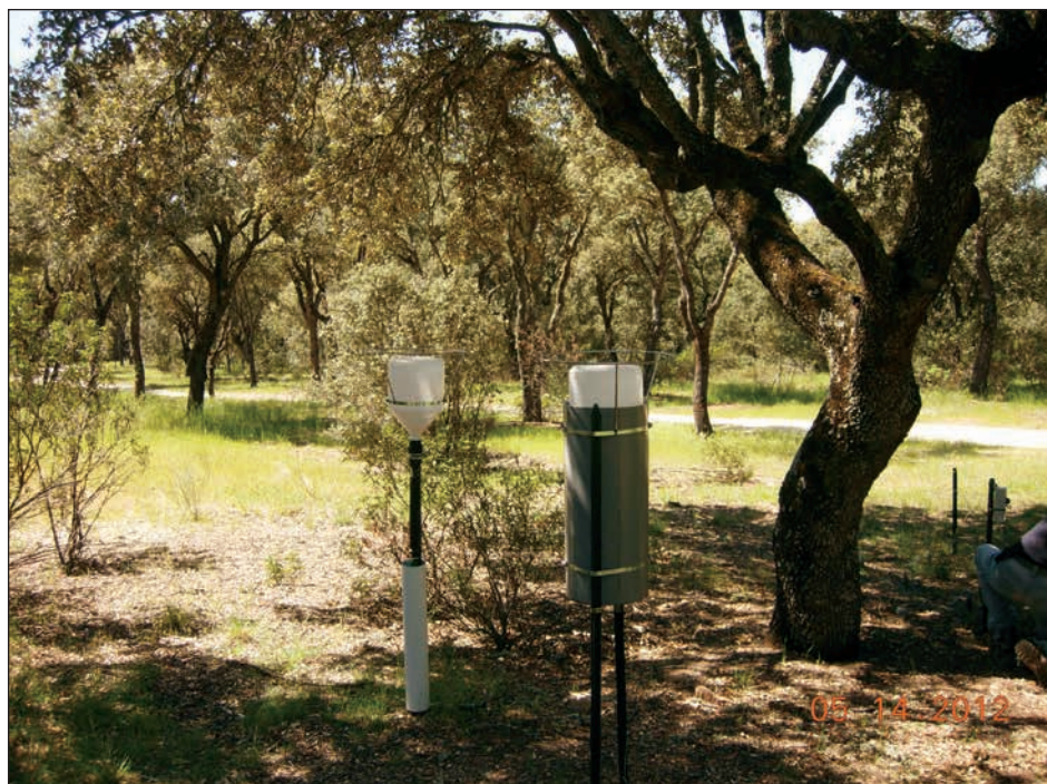
Figure 3.3—Ion exchange resin (IER) throughfall collector. Photograph is similar to figure 3.2 except that the shade tube covering the ion exchange resin (IER) column has been lowered to reveal the IER column. Also note the opaque cover over the liquid solution collector on the right to protect the sample from sunlight and reduce warming of the sampler.
