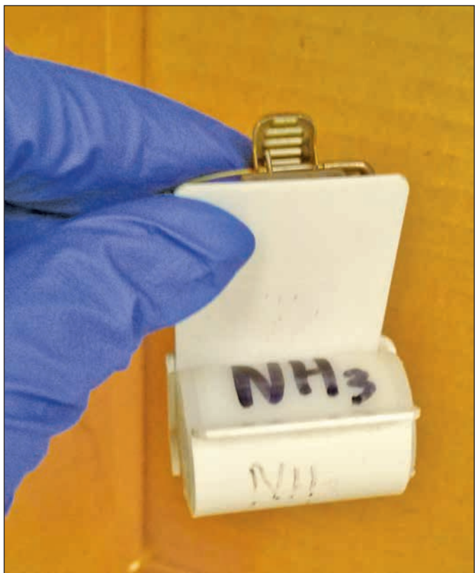
Figure A1.14—How to hold the Ogawa sampler by the clip.
