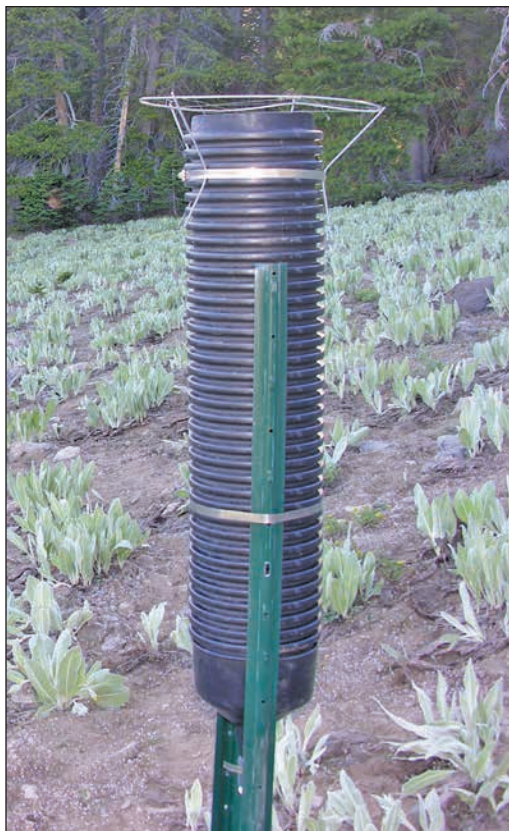
Figure 3.15—Ion exchange resin throughfall collector with snow tube inserted into the funnel. Snow tubes such as this one, about 1.0 m in length, are used in locations with high levels of winter snowfall.
