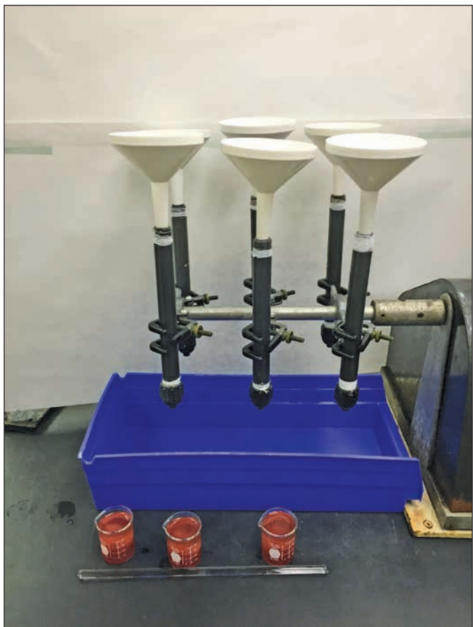
Figure A2.2—Ion exchange resin (IER) column and hardware used to fill the columns (top). Setup for filling the columns with IER beads (bottom).
