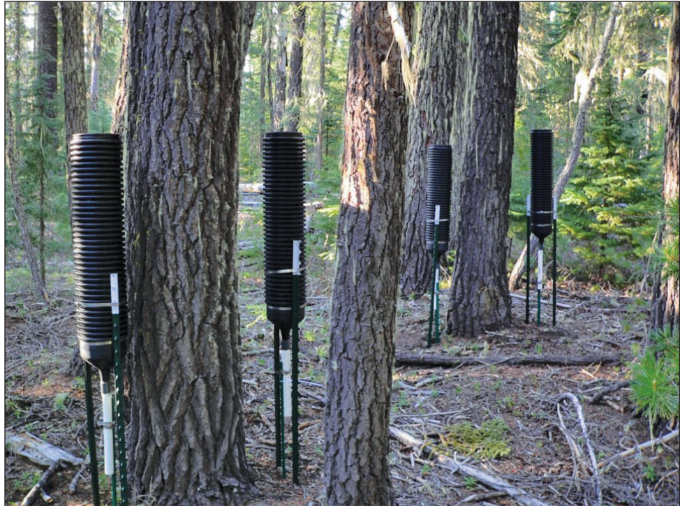
Figure 3.11—Installation of ion exchange resin throughfall collectors with snow tubes at a forest site. The tree canopy serves as the atmospheric deposition collector surface for throughfall samples that are washed from the canopy by precipitation or snowmelt.
