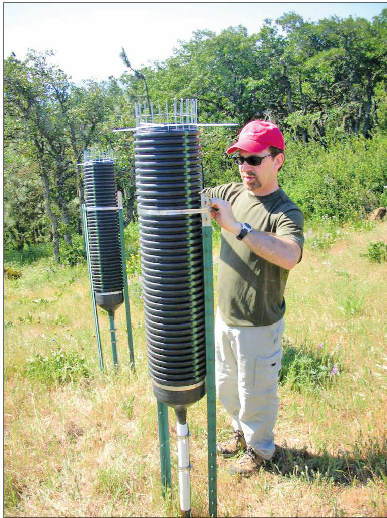
Figure A2.3—Ion exchange resin collectors installed in the field, showing the snow tubes as mounted onto fence posts and with a bird deterrent attached.
