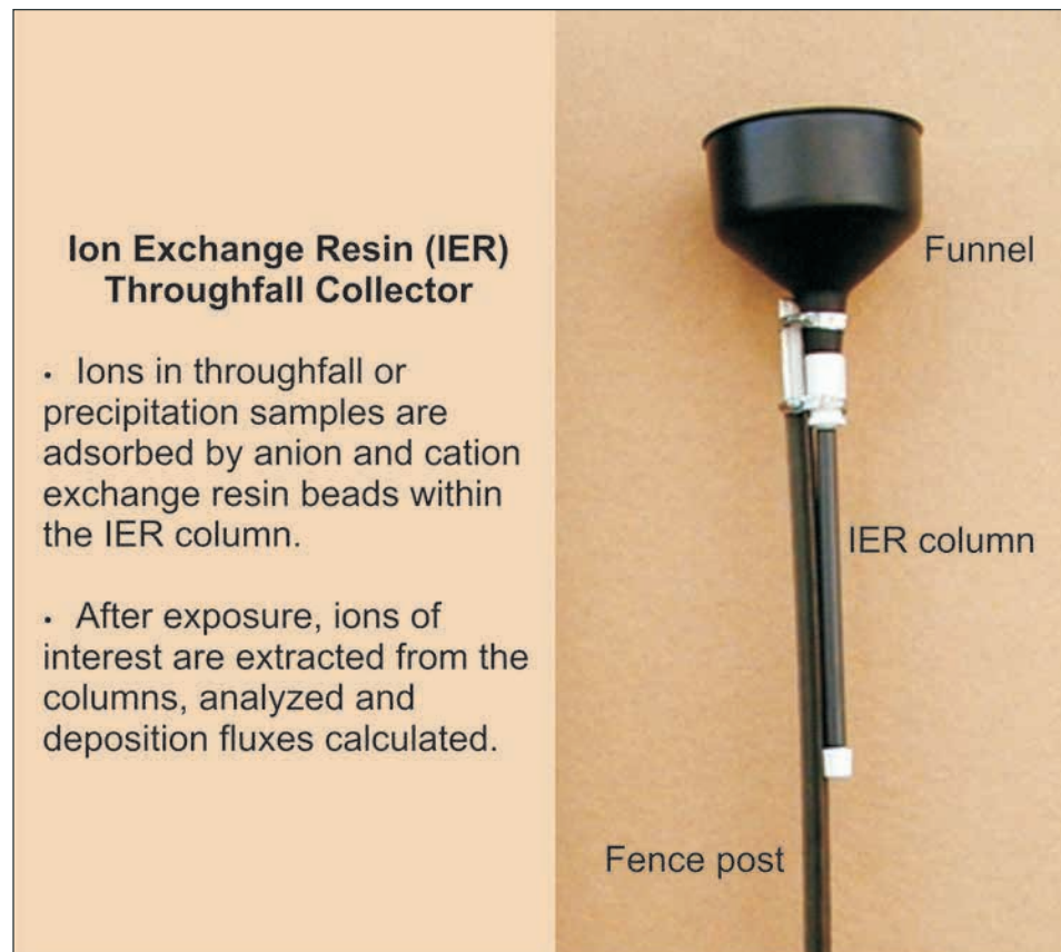
Figure 3.1—Photograph of an IER bulk deposition collector. Ion exchange resin collectors are used to collect precipitation (placed in open, canopy-free areas) or throughfall (placed under tree or other vegetation canopies) deposition samples.
