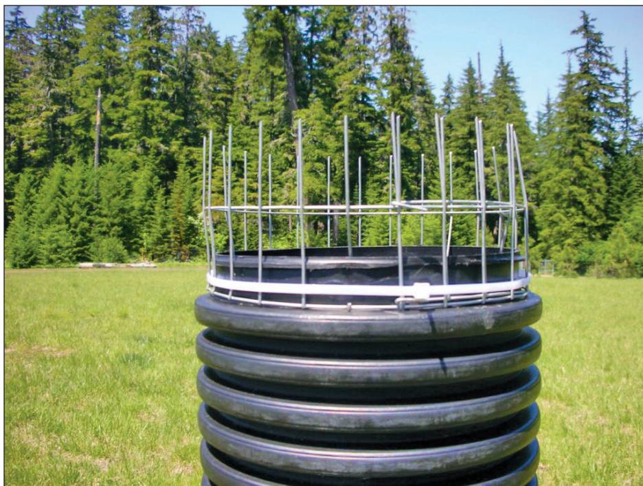
Figure A2.4—Closeup side view of a bird deterrent attached to a snow tube. Note that this bird deterrent is different than the bird sitting ring shown in figures 3.7 and 3.20.
