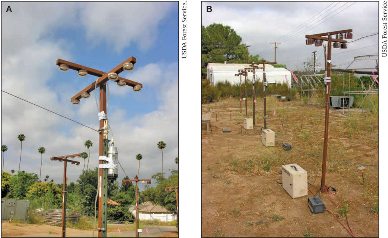
Figure 2.2—(A) Honeycomb denuder/filter pack system (active sampler unit strapped to the vertical post) used for calibration of ammonia and nitric acid passive samplers (mounted on the upper cross bars); and (B) a passive sampler calibration experiment at the Pacific Southwest Research Station Riverside Laboratory. Note that electricity is only required for the active samplers in the calibration, not the passive samplers.
