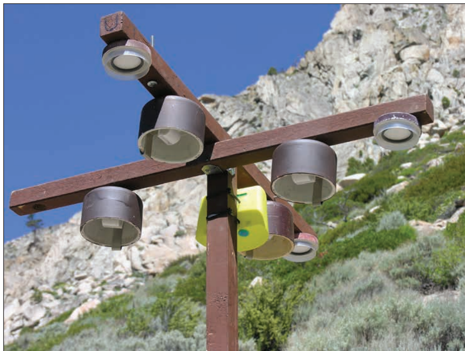
Figure 2.6—Closeup view of a setup for passive monitoring of multiple gaseous pollutants. The yellow housing unit contains passive samplers for volatile organic compounds (Burley et al. 2015), illustrating an additional type of pollutant that can be passively sampled.
