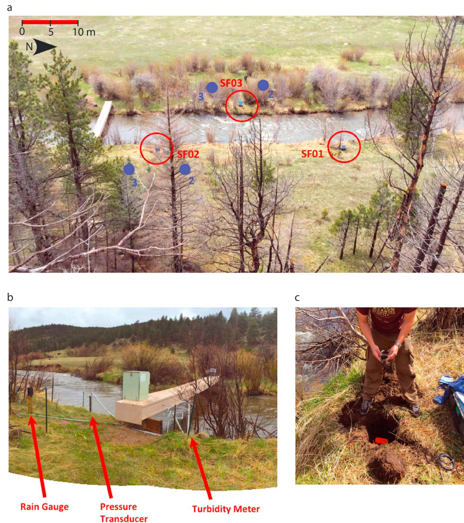
Figure 1. (a) Field site along a straight reach of the South Fork Cache la Poudre River, Northern Colorado. Seismic stations SF01–SF03 are shown along with infrasound sensors locations (blue circles, sensor 1 colocated with seismic stations, person for scale next to SF03 label). (b) Locations of rain gauge, pressure transducer, and turbidity meter. (c) Three-component Sercel L28 (4.5 Hz lower corner frequency) geophones were placed ~1 m from the channel and at water table depth just prior to rising limb conditions in mid-May. GPS-time-stamped data were recorded on solar powered Reftek RT-130 data loggers. This reach of the river runs nearly north-to-south, so that the north component of the seismometer is very nearly parallel, and the east component very nearly perpendicular, to flow, which is to the right (north) in Figures 1a and 1b.
