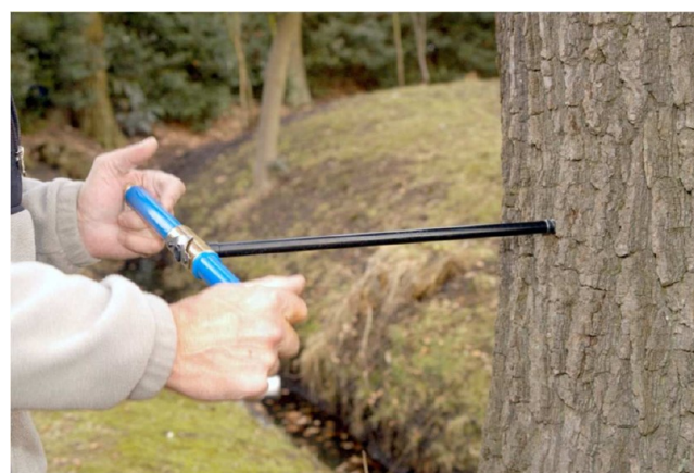
Figure 2. Sampling of tree 2 using a 10-mm Pressler borer.
