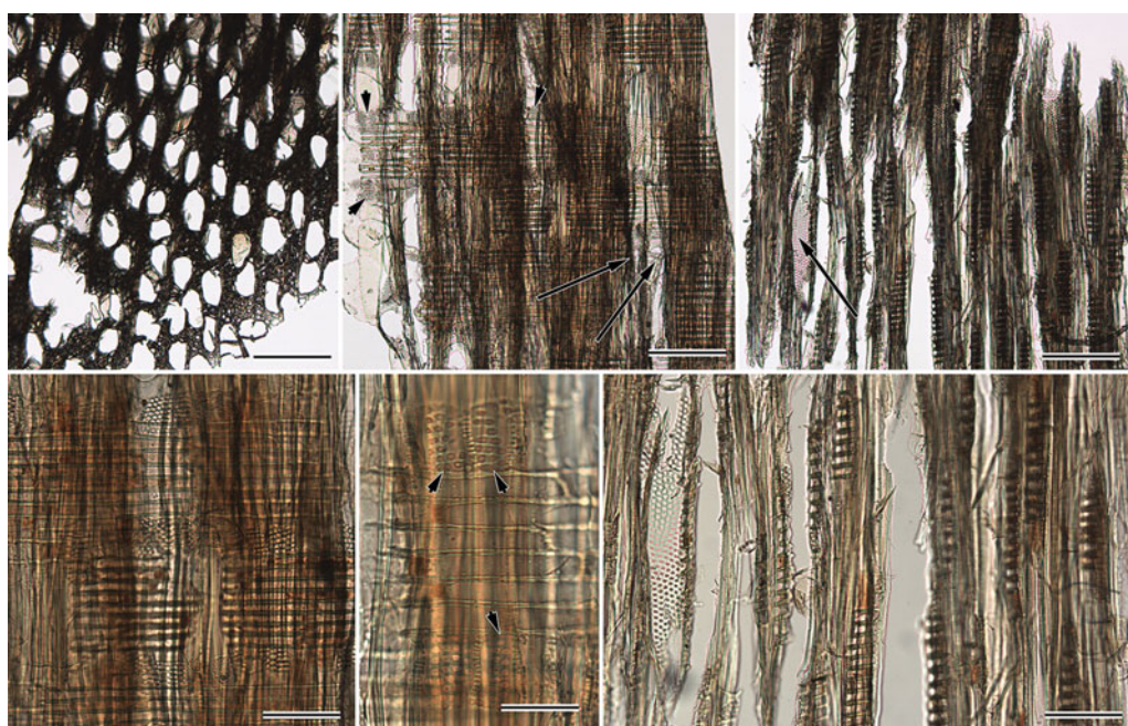
Figure 8. Transmitted light micrographs of the wood anatomy of the wooden base. Unless otherwise noted, all scale bars are 200 \mu\text{m} . Top left) transverse section showing diffuse-porous wood, abundant vessels solitary and in multiples of 2–3 and apparently narrow rays. Top middle) radial section showing simple perforation plates (arrows) and larger than ray-vessel pitting (arrowheads). Top right) tangential section showing uniseriate rays and alternate, medium-sized intervessel pits (arrow). Bottom left) radial section showing clear distinction between procumbent cells and upright cells, including disparate ray-vessel pitting (100 \mu\text{m} ). Bottom centre) radial section showing marginal upright cells (arrowheads), distinguishing between Salix and Populus (50 \mu\text{m} ). Bottom right) tangential section clearly showing uniseriate rays and alternate intervessel pits (100 \mu\text{m} ). Images: A.C. Wiedenhoeft.
