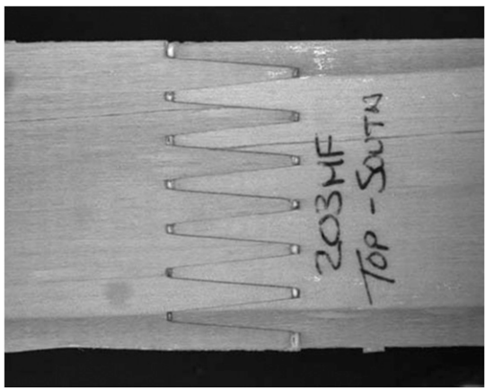
Figure 1. Representative finger joint made in the laboratory.
