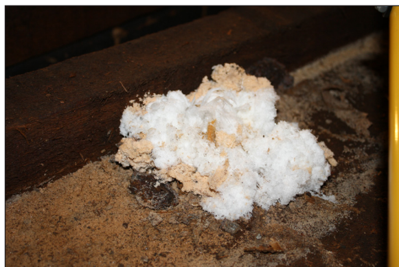
Figure 4. White corrosion product on top of metal fasteners in the forward bilge.
