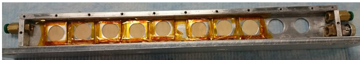
Figure A- 2 Humidity chamber showing samples held in place using polyamide tape.
