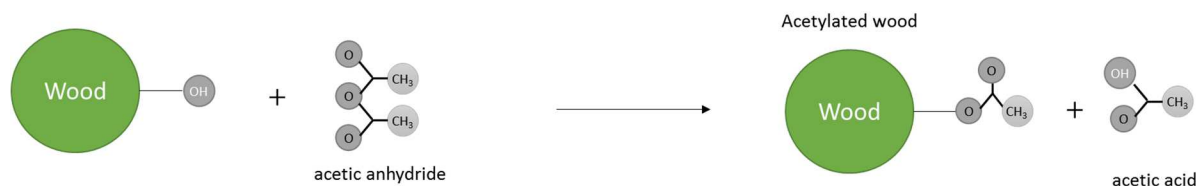
Figure 4.2 Schematic showing acetylation process including reactants and products.
