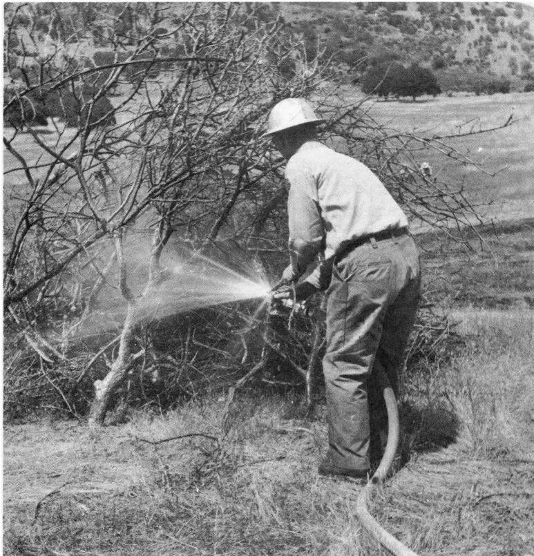
Figure 2.--Spraying viscous diammonium phosphate on end of a brush pile at the Mariposa field tests.
