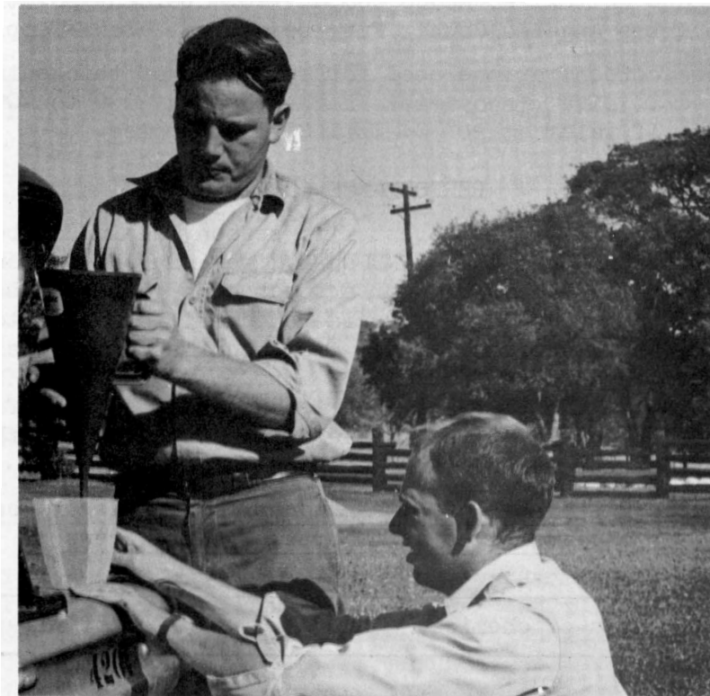
Figure 7 --Determining viscosity in the field with a Marsh funnel. The time required for the solution to run through the funnel gives an estimate of viscosity.
