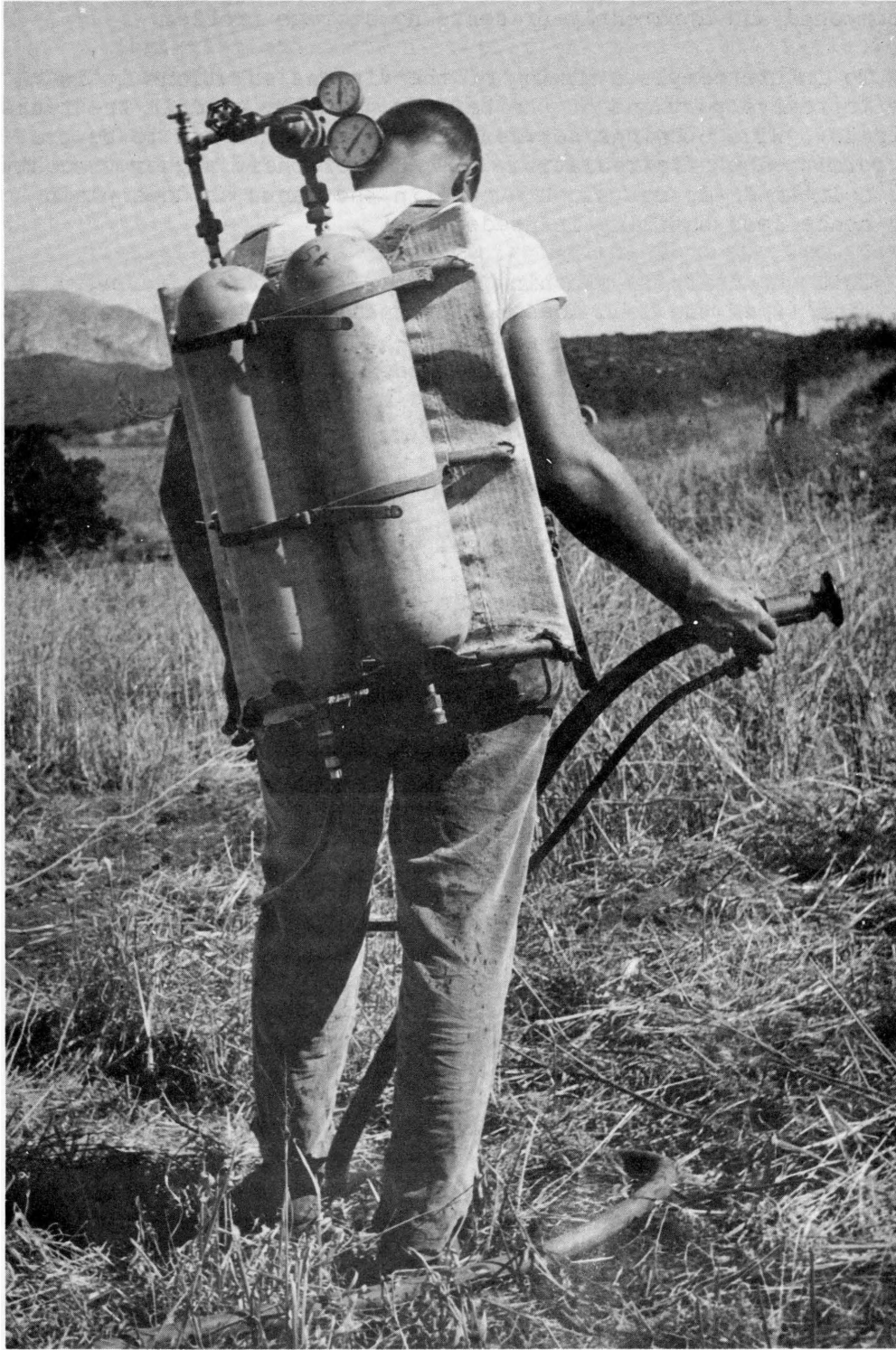
Figure 8.--Backpack arrangement and nozzle used to mix calcium chloride to algin to form calcium alginate gel.
