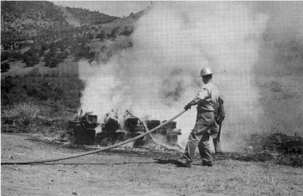
Figure 1.--Extinguishing a railroad tie crib fire with viscous water at a series of field tests held at Mariposa.
