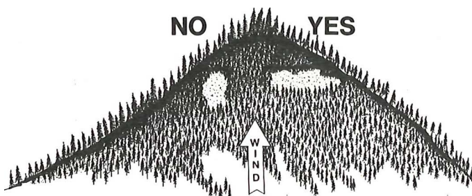
Figure 13.—Clearcut unit boundaries laid out across the slope that expose the short dimensions of the unit to the wind helps reduce blowdown.
