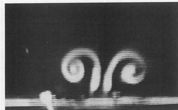
FIG. 12. A wind tunnel cross-sectional photograph of two pairs of horizontal vortices that formed over two longitudinally embedded nichrome wires. The photograph was taken with the camera positioned downstream at the tunnel exit at about a 10^\circ angle off the axis of the flow.
