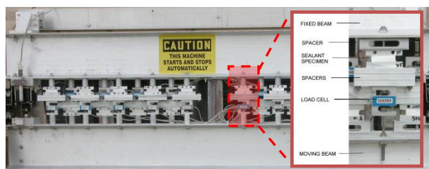
Figure 1: Photograph of mounted sealant specimens. The inset image is a close up of one assembly.
