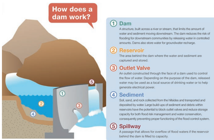
Fig. 7.1 Schematic diagram of a flood control dam describing different components (County of Los Angeles, Department of Public Works, www.lasedimentmanagement.com )
