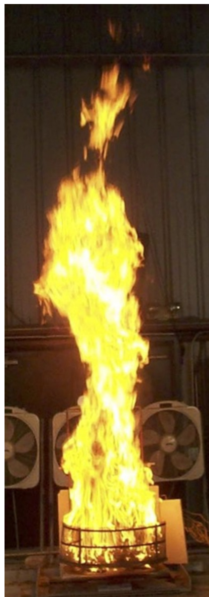
Fig. 1. Circular crib fire created by burning solid fuel composed of chamise branches and foliage.
