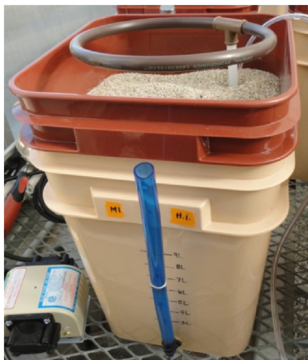
Fig. 1. Example of an ITNI module. The upper dark brown insert contains the quartz sand substrate in which the plants are grown. The brown water ring distributes water to the plants from the lower tan-colored reservoir when air is pumped from the small clear plastic tubing into the white plastic riser (i.e., an air-lift). The blue plastic tubing is used to measure the water level in the lower reservoir and to add deionized water to the module when necessary. (For interpretation of the references to color in this figure legend, the reader is referred to the web version of this article.)
