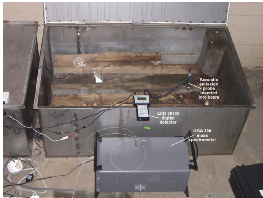
Figure 5. Termite boxes for testing AE signals to establish an AE fingerprint of R. flavipes invading red pine and Southern Pine members.
