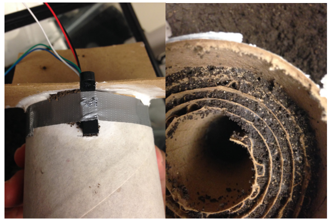
Figure 12. LED light sensor set to maintain 0 V as long as detector receives light.
