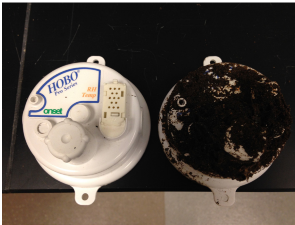
Figure 11. Termite mud/shelter tube deposition by termites on the plastic surface of sensor.
