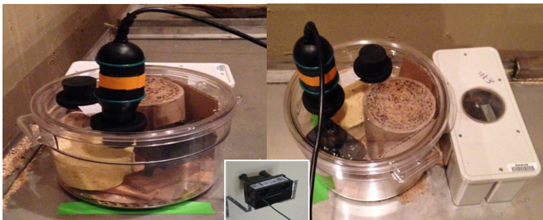
Figure 15. Two external, aboveground termite bait stations, each containing the OmniSense Remote wireless sensor (inset), which tracks RH and temperature 24 h per day as termites in the parent tank accept these bait stations into the colony domain and begin to consume the substrates. Data can be downloaded from the internet and graphed.
