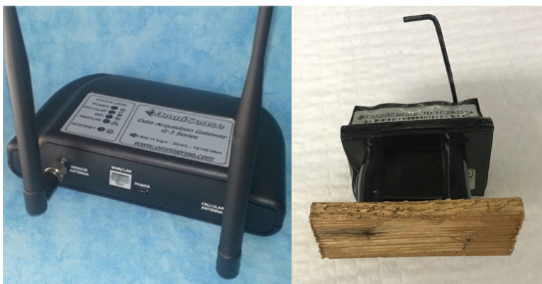
Figure 21. OmniSense Cellular gateway (left) and WME block with wireless antenna (right).
