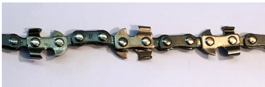
Figure 5— Specialty saw chain (PockeTech HighLimb2-48 inch) that has bladed chisels on both sides of the chain and in both directions. (Photo by John Butnor)
