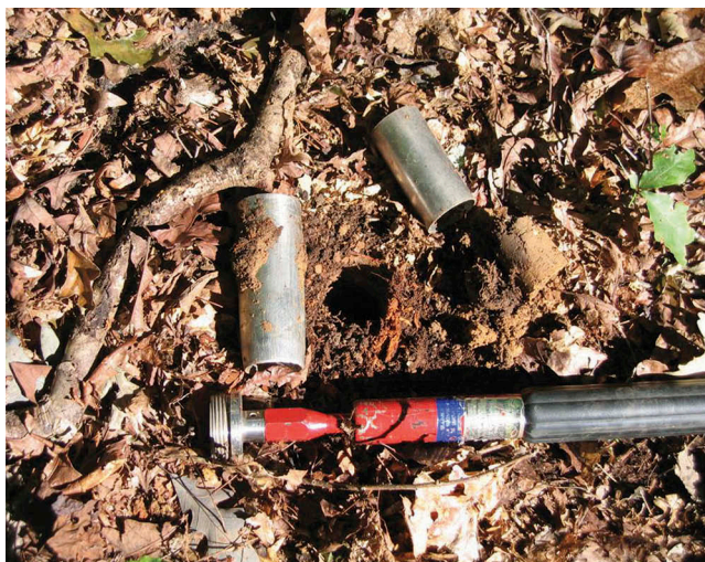
Figure 1. The AMS Inc. Slide Hammer used for sampling soils within the Cecil-Lloyd-Madison Association on the Clemson Experimental Forest, Clemson, South Carolina.
