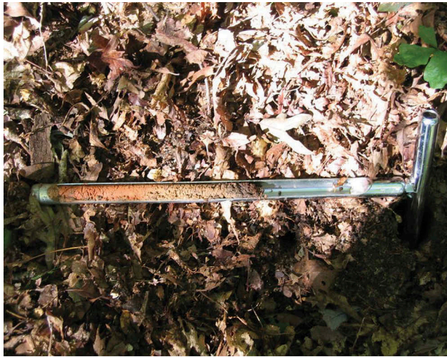
Figure 2. The Oakfield Model H Soil Probe used for sampling soils within the Cecil-Lloyd-Madison Association on the Clemson Experimental Forest, Clemson, South Carolina.
